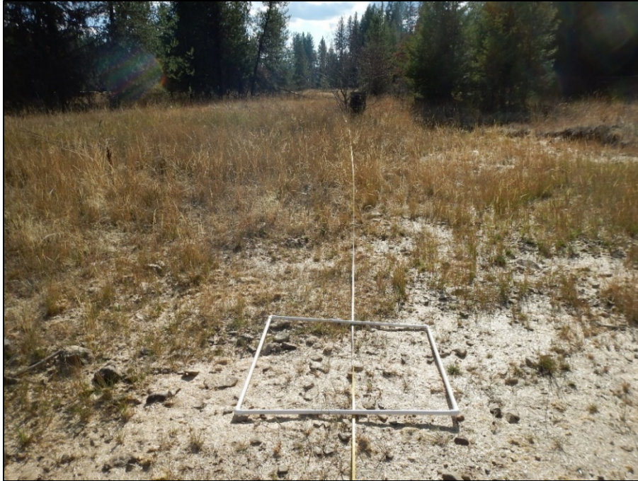
Figure 22. Racetrack Meadow, Transect 3, October 22, 2015 (2 years post-construction). Note seeded and mulched areas in the foreground as revegetation process continues. Taller grasses in the background are native perennial grasses seeded directly following construction in fall 2013. Most vegetation visible is meadow barley ( Hordeum brachyantherum ).
